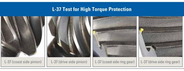
The test simulates an extreme load and high pressure operational environment inside a hypoid axle typical of a large truck. Low-speed, high torque operating environments lead to anomalies like abrasive wear, adhesive wear, plastic deformation, and surface fatigue. These conditions eventually can lead to gear and bearing failure, if left unprotected.
