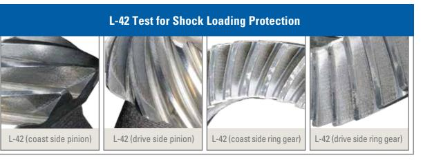
The test simulates a truck operational environment characterized by high speed and shock loading within the drive axles. This type of environment occurs in vehicles where abrupt accelerations and decelerations are common. The high speed and shock loading often leads to scoring on gear surfaces.
